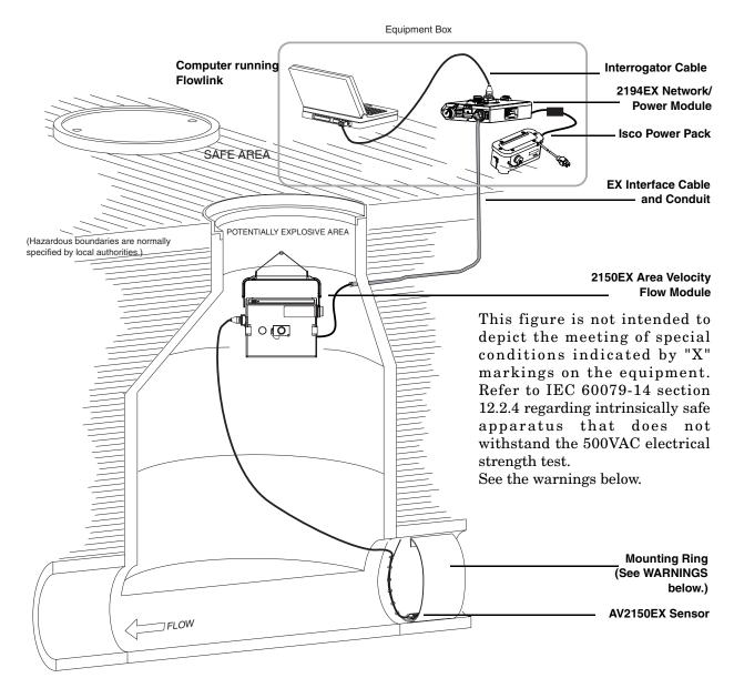
Figure 2-3 Typical Round-pipe Installation Connected to a 2194EX Module and Laptop (Permanent Installation, see section 2.5)
